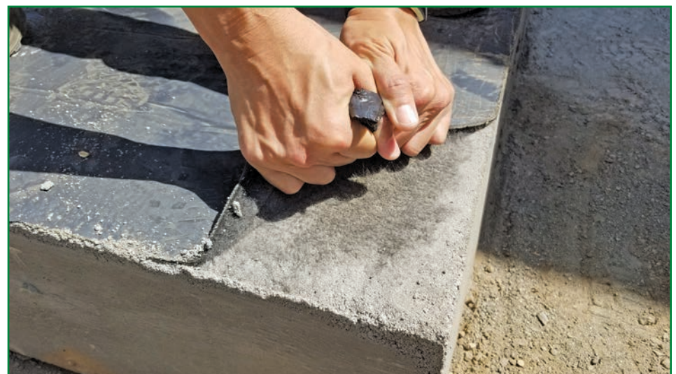
Figure 9 – Pull test of the waterproofing membrane by hand on a smaller 4- x 4-ft. mock-up.
